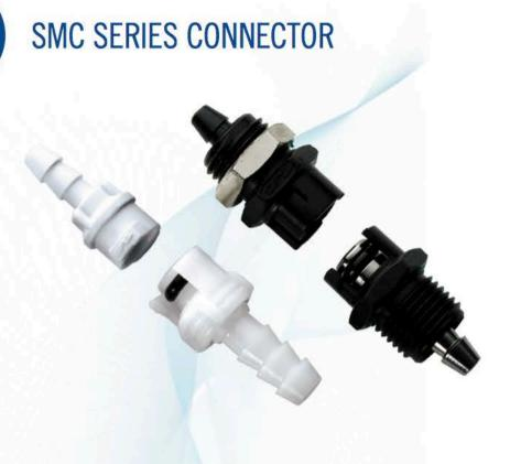
The SMC and SMF1 are among CPC's smallest couplings. These twistto-connect couplings provide a reliable and more secure alternative to luer-type connections. They also allow for the tubing to rotate freely when connected. This important feature prevents both kinked tubing and accidental disconnection during use.
